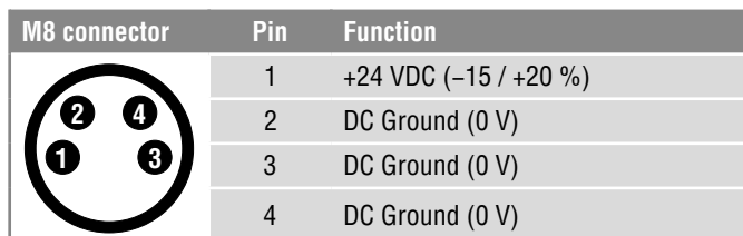
Fig. 74: Wiring for sensor reset step one.
